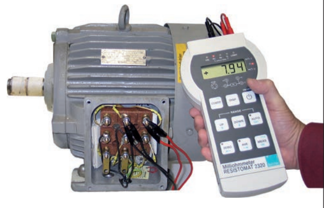
Coil winding measurement on a motor
