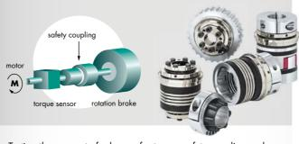
Testing the moment of release of a torque safety coupling under dynamic load.
