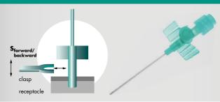
Testing the ease of movement of a venous canula over the length of the steel insertion needle. The clasp holds the canula and moves it up and back over the needle.
