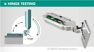
Measuring the correct torque/angle response in final testing of hinges.
