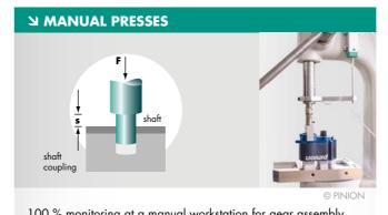
100 % monitoring at a manual workstation for gear assembly.
