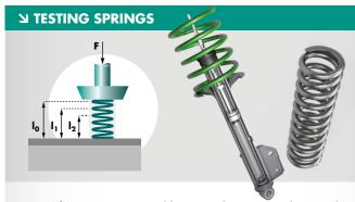
Testing of spring constant and hysteresis between applying and removing load.
