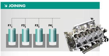
Multichannel monitoring of joining process in cylinder head assembly. The synchronous process during the assembly of valve seating rings and valve guides is measured and analyzed. DigiControl PC software logs and visualizes the process data from up to 32 controllers.
