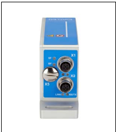
Fig. 17: View page with LEDs for PROFINET
