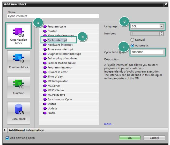
4. Type in the following source code in the code field of the new block:
