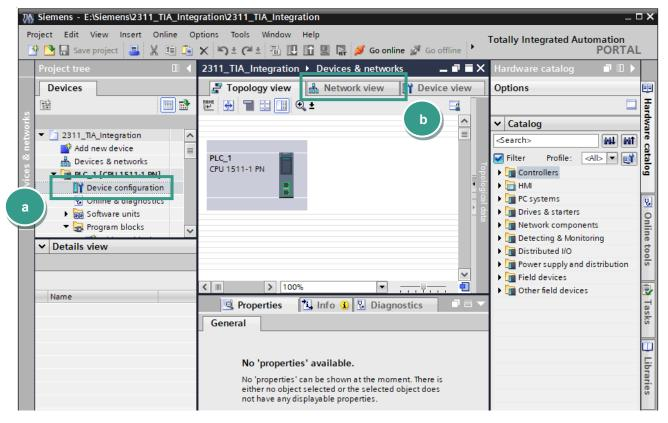
2. Now select the Resistomat 2311 device in the catalog and drag & drop it into the working area (a):
