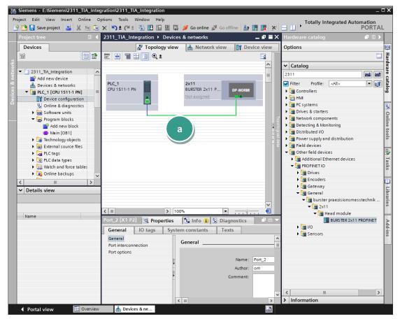
4. Change now to **Network view** (a) to assign a controller to the Resistomat 2311. Click on the link "Not assigned" (b) of Resistomat 2311 and select your controller (c):
