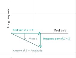
An alternating current  $I_{AC}$  is imposed in the test object and measures the resulting voltage drop  $U_{AC}$ . The AC voltage measurement takes place selectively and synchronously, with results in accordance with the real and imaginary part. The complex impedance (Z) is obtained by means of mathematical calculations. The real part represents the ohmic component, and the imaginary part represents the capacitive/inductive component.
