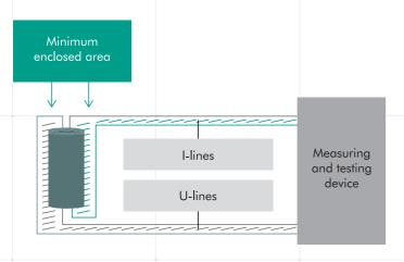
Inaccurate test object contacting, variable press-on force or geometry/surface/material of the contact pins also have a decisive part to play with regard to reproducible measuring results.
