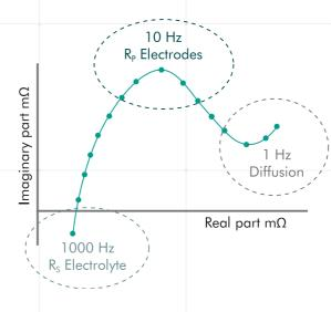
Spectral impedance measurement, result display in Nyquist diagram locus curve
