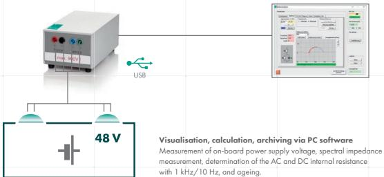
The open circuit voltage and the complex internal resistance between 1 Hz and 1 kHz must be determined on a 48 Volt on-board power supply battery, from which the status variables of ageing, charge condition and AC and DC internal resistance are to be mapped. Capacitive residual components can be determined without complicated discharge measurements in this way.
