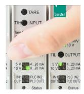
7 If you do not press the [TIL / OUTPUT] button for a second time within 3 seconds, the selection LED stops flashing and no change is made to the settings..
