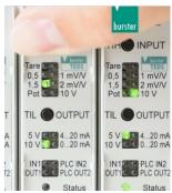
If you do not press the [TIH / INPUT] button for a second time within 3 seconds, the selection LED stops flashing and no change is made to the settings.
