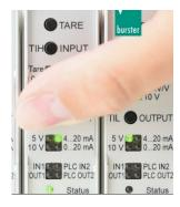
To adopt the currently made selection for the analog output, press and hold the [TIL / OUTPUT] button for about 3 seconds
