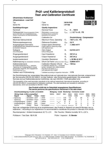
Diagram: 33 Test and calibration certificate for a strain-gage sensor (specimen)
