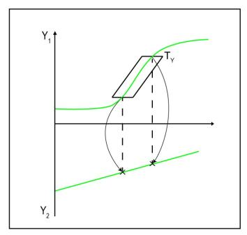
Diagram 38: Example for a trapezoid window – determining the resultant  $Y_2$ -values at the entry and exit points of the  $T_V$  evaluation element (Y-trapezoid enabled on curve  $Y_1(x)$ )
