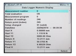
4 Select an active evaluation element and press [Enter] to display the OK/NOK result and additional values.
