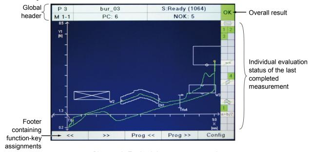
Diagram 56: Top-level view measurement results
