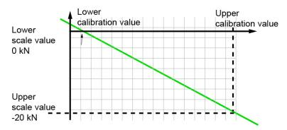
Diagram 28: Inverting measurement signals
