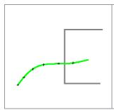
The DIGIFORCE® 9307 linearly interpolates the window entry coordinate from the last measurement point outside the window limits and the first measurement point inside the window limits
