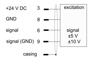
The +24 VDC transmitter supply can be switched on/off in the "Channel settings" menu.
