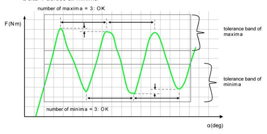
Diagram 13: Rotary switch evaluation
