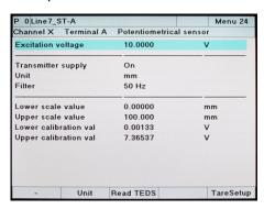
If the device detected a potentiometric sensor programmed with burster TEDS, it displays the "TEDS Info" function [F4].
