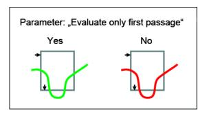
Specify whether the evaluation window is active on channel  $Y_1$  or  $Y_2$ . That completes the basic configuration of the evaluation window. In the "Advanced" section you can activate additional parameters for recording extra information.
