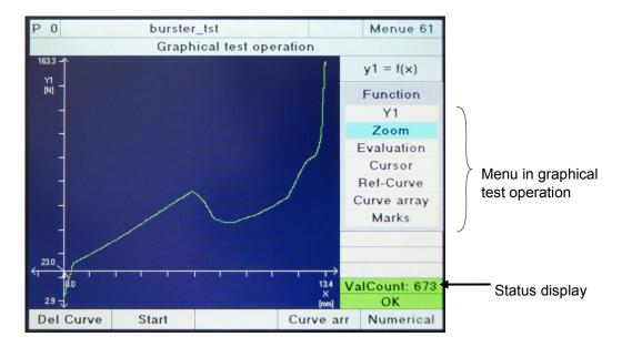
Diagram 48: Graphical test operation
