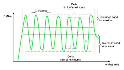
Diagram 44: Rotary-switch testing
