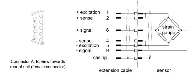
Make the connections between the sense lines and excitation lines as close as possible to the sensor.
