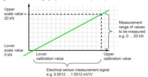
Diagram 27: Scaling of analog sensors
