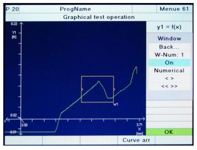
Diagram 49: Graphical test operation - Configuring windows
