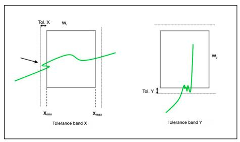
Diagram 45: Tolerance band for evaluation elements
