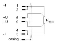
Note: In the 200 m $\Omega$  range, use two dual conductors of large cross-section to connect the "+1" and "-1" excitation to  $R_{meas}$  t.
