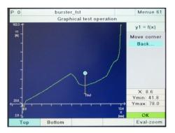
Pressing the **[Enter]** button completes the graphical configuration process for the threshold. In the Numerical submenu you can now specify the direction in which the measurement curve crosses the threshold plus any other parameters relating to the Threshold element (see section 6.8.5 "Threshold" on page 131).
