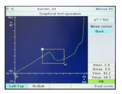
Pressing the **[Enter]** button completes the graphical window configuration process. In the "Numerical" submenu you can now specify the entry and exit sides of the window plus other parameters relating to the "Window" evaluation element.
