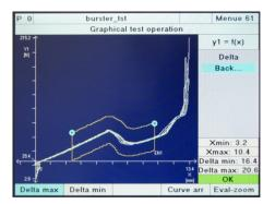
That completes the envelope generation process. In the "Numerical" submenu you can make numerical adjustments to the values you have set graphically such as the start and end positions. Press [ESC] to exit the menu.
