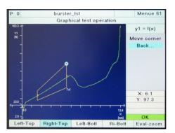
Pressing the **[Enter]** button completes the graphical configuration process for the trapezoid window. In the Numerical submenu you can now specify the entry and exit sides of the trapezoid window plus any other parameters relating to the trapezoid window element ( see section 6.8.3 "Trapezoid window" on page 125).
