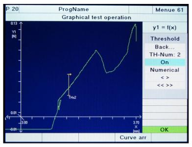
Diagram 51: Graphical test operation - Configuring thresholds
