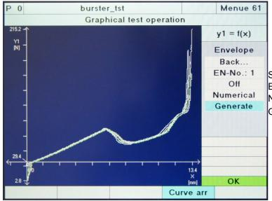
Selecting envelope 1 or 2 Element On/Off Numerical configuration Generate envelope
