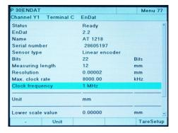
5 Close the Channel setup menu and confirm the settings with [ENTER].
