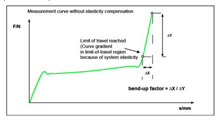
Diagram 32: Finding the bend-up factor from a real measurement curve
