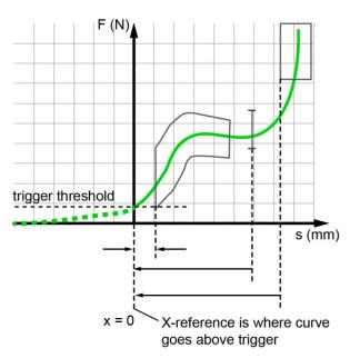
Diagram 11: Measurement curve with TRIGGER reference (example)
