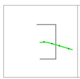
The DIGIFORCE® 9307 linearly interpolates the window exit coordinate from the last measurement point inside the window limits and the first measurement point outside the window limits.
