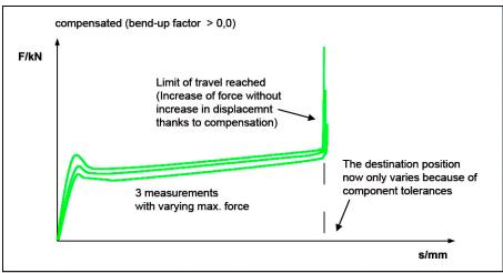
Diagram 31: Example ball bearing
