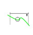
The DIGIFORCE  $^{\circ}$  9307 finds the **first** local maximum of the Y-coordinate within the span of the type-Y threshold and outputs the coordinates as an X/Y value pair.
