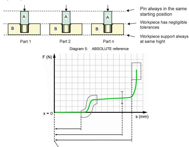
Diagram 6: Measurement curve with ABSOLUTE reference (example)
