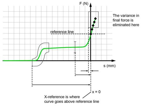
Diagram 9: Measurement curve with REFERENCE LINE reference (example)
