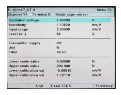
If the device detected a strain-gage sensor programmed with burster TEDS, it displays the "TEDS Info" function [F4].
