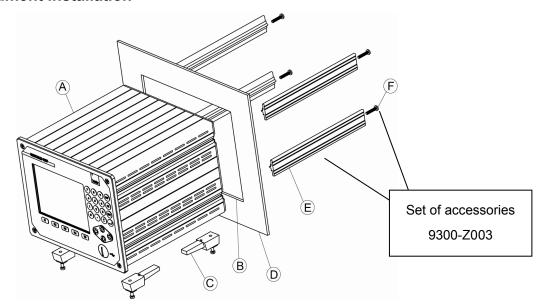
Diagram 20: Instrumen installation
