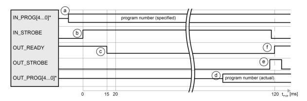
\* IN\_PROG[6..0] and OUT\_PROG[6...0] for 128 measurement programs. You can define a user-configurable PLC output for the signal "OUT\_PROG[6..0]".
