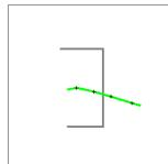
The DIGIFORCE® 9307 linearly interpolates the window exit coordinate from the last measurement point inside the window limits and the first measurement point outside the window limits
