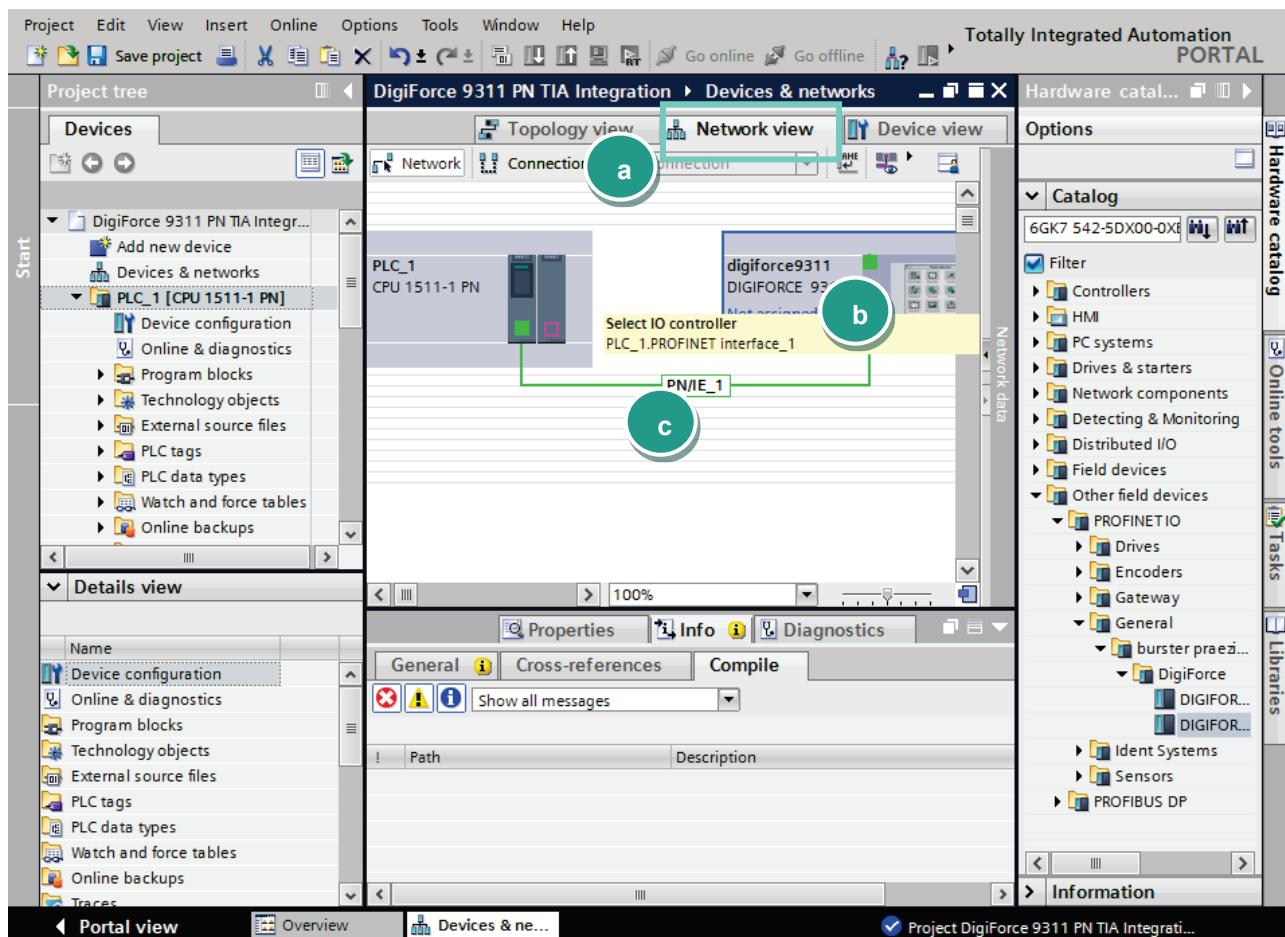
Check if devices also connected physically to the right ports. You find the port number assignment in the section **4.3 Port-Identification of DIGIFORCE® 9311 PROFINET** manual
