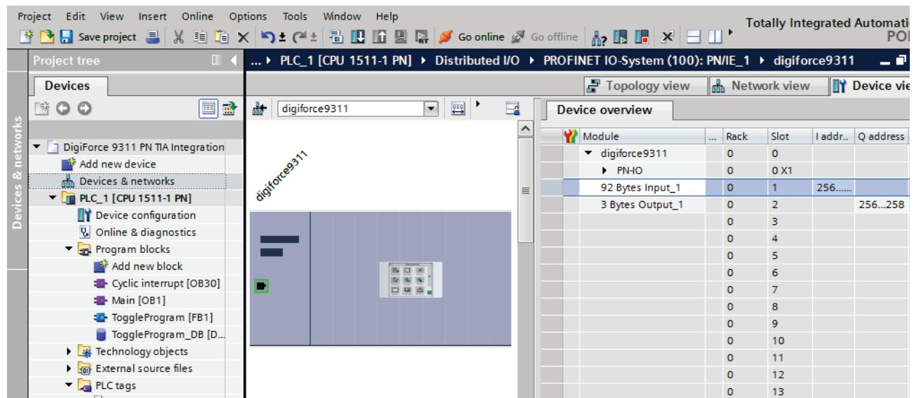
You will also see that the TIA-Editor replaces the input/output addresses with tags. You can change the tags names in PLC Tag table (e.g. to IN\_START and OUT\_READY):
