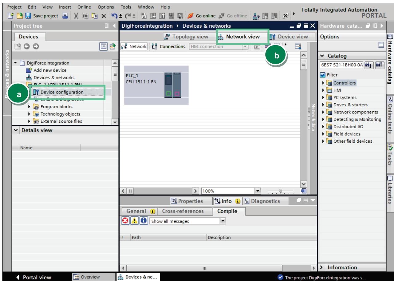
➤ Now select the DIGIFORCE® 9311 device in the catalog and drag & drop it into the working area (a):
