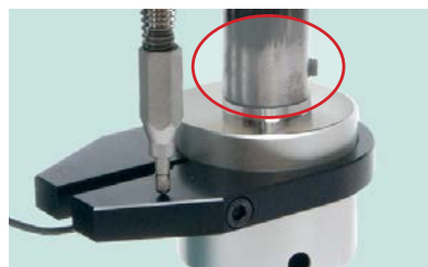
Ram with internal bore and grub screw
