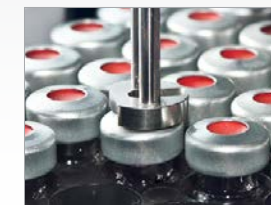
Press-fitting sealing plugs
