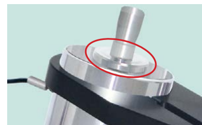
Load cell contact area, via which force is transmitted
