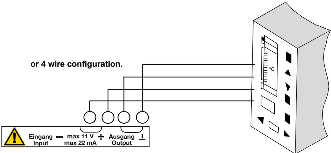
Switch on the device and connect it as shown above.
