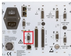
Figure 1: Communication via RS232
