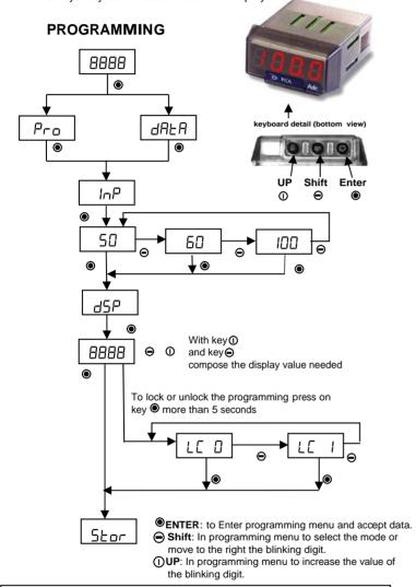
InP: Programming of shunt type used. 50 mV, 60 mV or 100 mV dSP: Programming of shunt nominal value. Example: with a 100 A / 60 mV shunt display is programmed to display 100 and automatically when the value is accepted the displayed value will turn to be 100.0. When a display value < 200 is programmed the value will be with a decimal and when a display value > 200 is programmed the value will be without.
