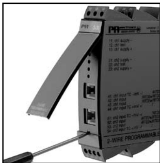
Picture 3: Access to programming connector.
