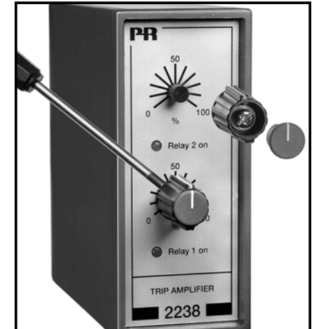
Picture 2: Removal of knobs.
