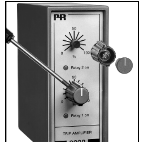
Picture 2: Removal of knobs
