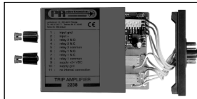
Picture 3: Removal of PCBs for adjustment of dipswitches and replacement of jumpers.
